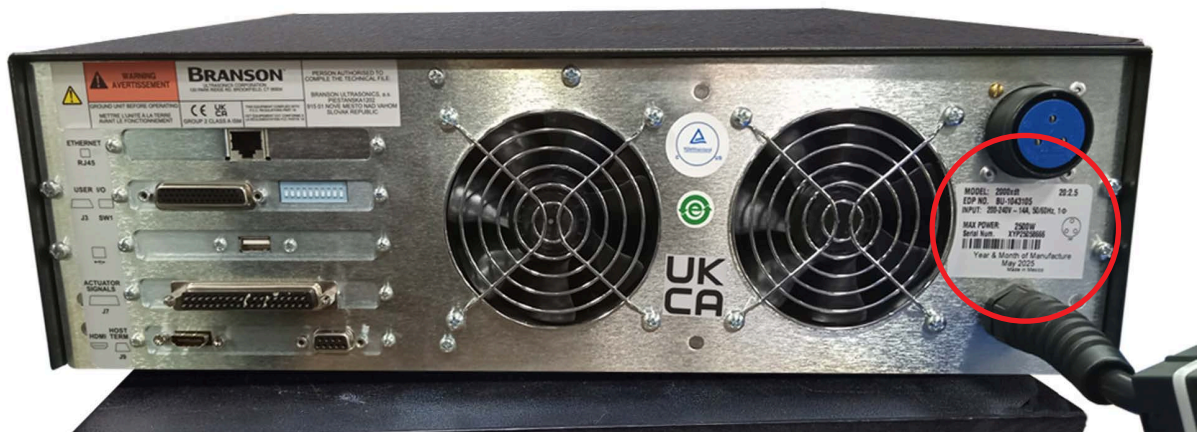
Figure E.1 Location of the information Label in the 2000Xc Power Supply
