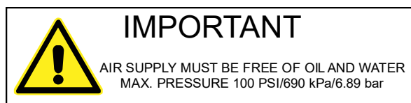
Figure 1.2 Caution label on the 2000Xc Series Actuator for the factory air supply
