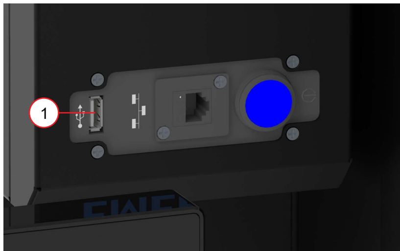
Figure F.8 Power Supply - USB port on the GSX-E1 system
