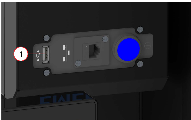
Figure 4.25 Power Supply - USB port on the GSX-E1 system
