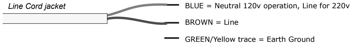
Figure 4.13 International Harmonized Line Cord Color Code
